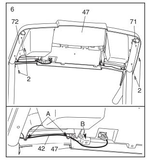
7. Cover the Upright Wire (42) with the Right Grip Plate (36). **Be careful not to pinch the Upright Wire.** Tighten a 3/4" Screw (2) and two 1/2" Screws (48) into the Right Grip Plate and the Console Base (47).
